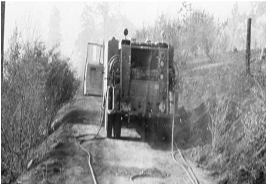
Jerseydale tanker after burn over...note the fuels on both sides of Ponderosa Way Hose lines were deployed due to tanker only being able to pump while stationary
